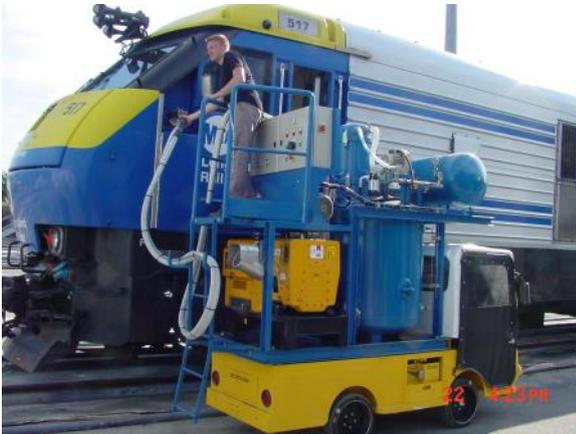
The **MOBISAND NEU – HMU type** is a mobile unit for filling all types of locomotive sand boxes, completely independent during the filling operation. It can be used alone or in addition to a fixed sand feeding installation in hard-to-reach areas. It is particularly suited for filling big sandboxes (sand flow from 20 to 40 l/min).
